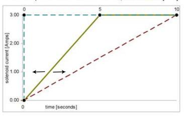
rdn: RAMP DOWN, Time for Output to Decrease from max to min, 0.0 to 99.5 [SEC]
